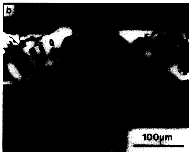
Figure 13 TOM micrograph of the sub-surface damage zone in epoxy toughened by 10 vol% HLP-15 particles viewed under (a) bright field and (b) cross-polars. Thin sample is taken from the mid-plane of a 3PB specimen. Crack growth direction is from left to right
